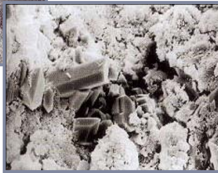
Microscopic view of Sulphate crystals in concrete
