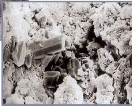
Microscopic view of Sulphate crystals in concrete
